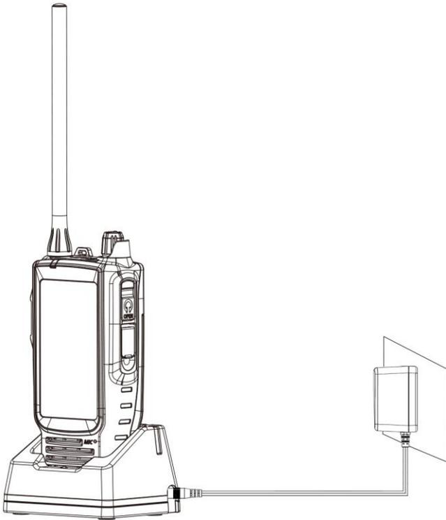
Figure 2 - TS19 AC/DC adapter and charge base
