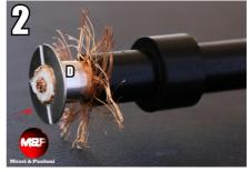
Insert component D after having opened the braid as shown in the picture. Push component D between the foil and the braid until it stops against the black PVC jacket.
