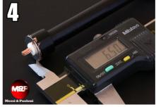
Cut and remove the tape and dieletric for a length as shown in the picture (6mm).
