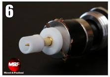
Insert the teflon tube as shown in the picture.
